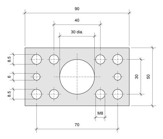
PLATE REFERENCE: **PL00** WELD TO BEARING: **4.053** USE WITH STEEL CHANNEL: **EC053**
